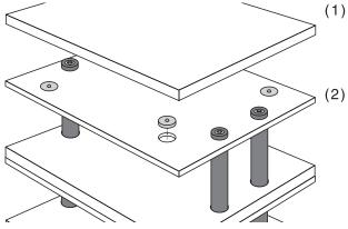
Insert the shelf board support spikes (8) into the recesses on the holding board ②, with the pins facing up (4 places).
