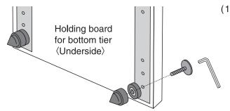
(1) Place the holding board for the bottom tier ① vertically on the floor. Pass the assembly screw for bottom tier ⑩ through the leg spike mounting hole. Mount the leg spike lock nut ⑪ on the screw and tighten it by hand to hold the screw snugly against the board without clearance. Finally, use the hexagonal wrench ⑭ and firmly tighten the screw. Having set the screw ⑩, thread the leg spike ⑫ on the screw ⑩ and tighten until it closely contacts the lock nut ⑪ (repeat for all 4 leg spikes).
