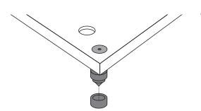
(2) Having installed the 4 leg spikes ①, lay down the holding board ① flat on the floor in the correct direction and insert the leg spikes ② into the spike receivers ③.
